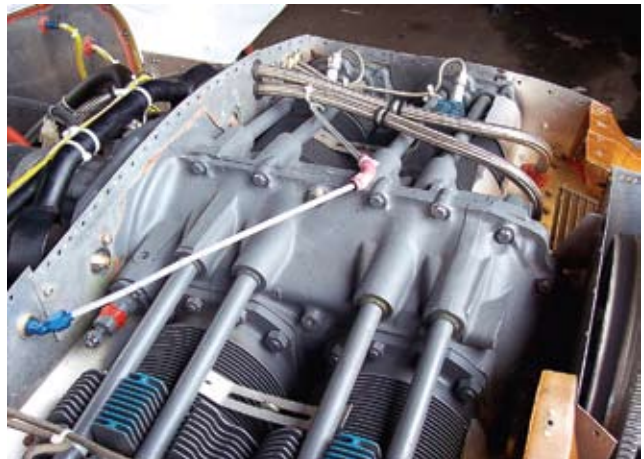
Piccolo tube used to measure static pressure above the engine. Additional probes are located below the cylinders and at the cowl exit.
