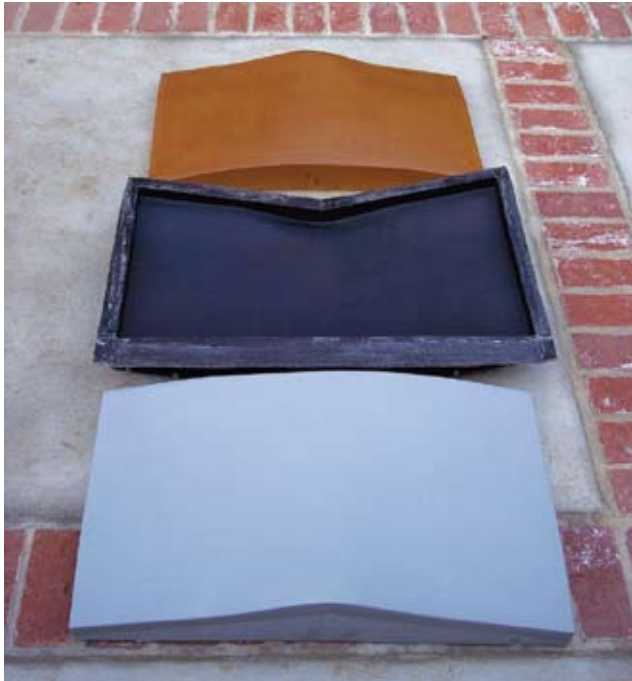
Plenum Top: plug, mold and finished part.
