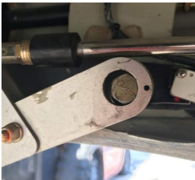
Figure 2, An Over-Center link that slipped off the bearing
