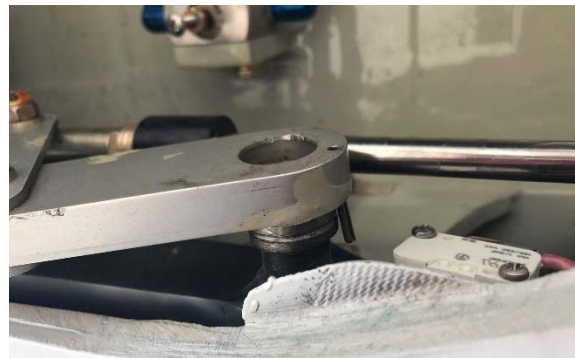
Figure 2, An Over-Center link that slipped off the bearing
